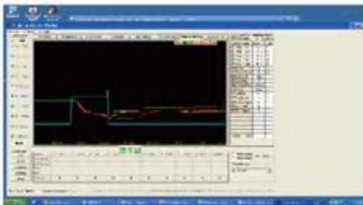
In start up & maintenance, software can connect with outdoor unit by TD-01, read all indoor unit & outdoor unit running parameter, also with the function to show parameter curve.
