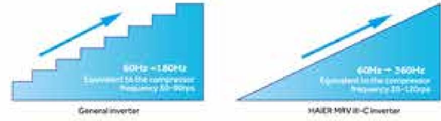
180° vector, dc inverter drive technology. Sine wave current drive, efficiency improve 17% comparing to conventional rectangle wave.
